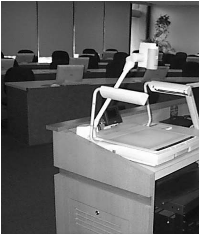
Figure 2. Instructor's station showing audio-visual controls, document reader, VHS, DVD and computer controls.
