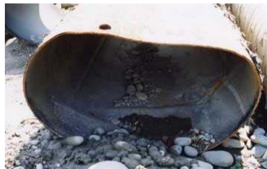
Figure 4. Large deformation of steel pipe section crossing the active fault (The 1999 Chi-Chi Earthquake in Taiwan)
