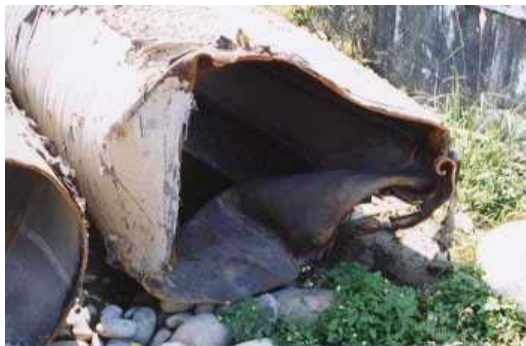
Figure 4. Large deformation of steel pipe section crossing the active fault (The 1999 Chi-Chi Earthquake in Taiwan)
