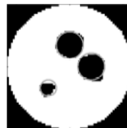
Fig. 3 Reconstruction of three 'bubbles' using an adapted ART algorithm.
